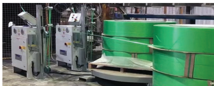
Detail of motorized storage dispenser and turntable
